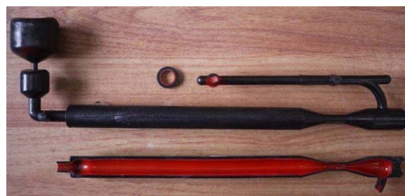
Figure 3. Overflow WACIM specimen. [Color figure can be viewed in the online issue, which is available at wileyonlinelibrary.com.]
